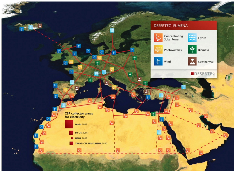
Figure 2.4: Sketch of possible infrastructure for a sustainable supply of power to Europe, the Middle East and North Africa (EU-MENA) (Euro-Super grid with a EU-MENA-Connection proposed by TREC) [34].
